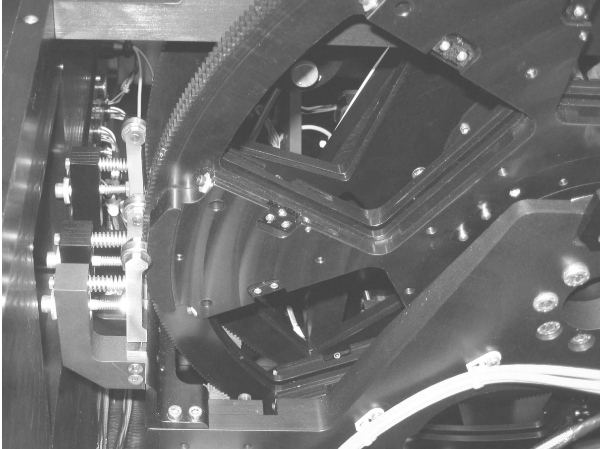
Figure 6. A closeup of filter wheel 2. The detent is the structure on the left side. Behind it are the detents for filter wheel 1 and the disperser wheel.
