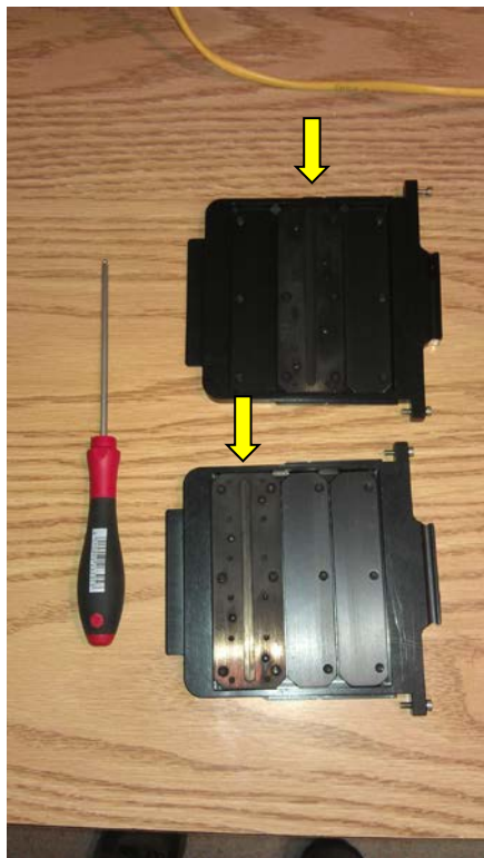
Figure 36: Longslits in holders (left). The slit holders shown are for a centered slit (top) and a blue-displaced slit (bottom), marked by the arrows. The red-displaced slits have the slit in the position near the handle of the holder. Slit mask mounted in wheel.
