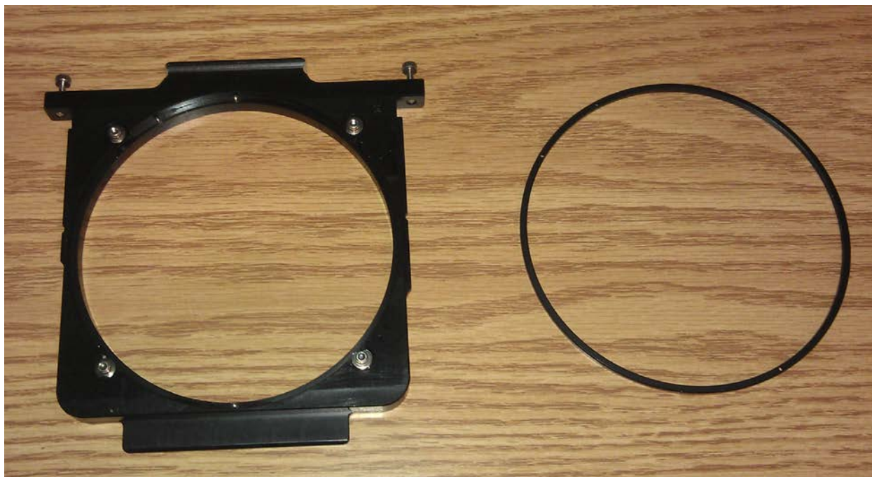
Figure 33: Mask holder with retaining ring removed . The 4 clamps can be seen around the inner edge of the holder. Alignment pins can also be seen at approximately the 6, 11, and 12 o'clock positions.
