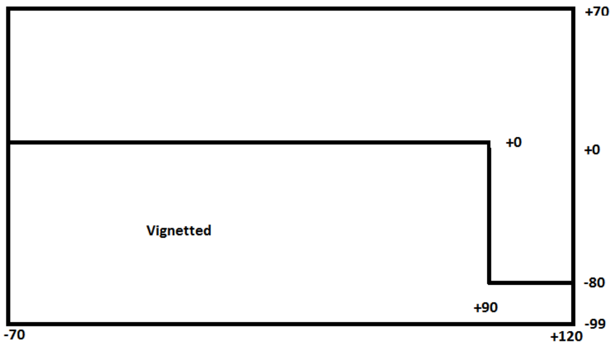
Figure 25: Blanco guider patrol area relative to the COSMOS field of view. Selection of guide stars within the lower region can cause the guide probe to vignette the COSMOS field. The size of the region that leads to vignetting is somewhat conservative, particularly for longslit spectroscopy.
