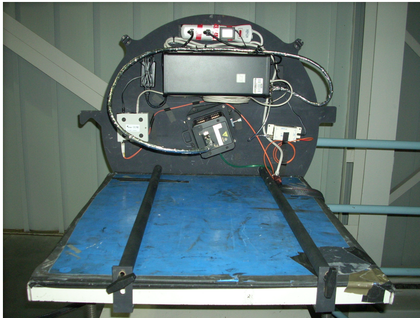
Figure 1: Agile on its cart: The CCD camera is attached to an assembly at the center of the mounting plate. On top of the CCD camera and attached to it with a triple-shielded analog cable is the electronics controller.
